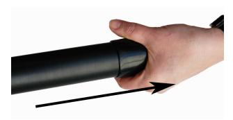
Open the lever on the extension and slide it on from the base of the pole. Fully side the section up the pole and close the clamp lever. You will need to slide the pole hose up from the base of the pole and re-connect to the gooseneck before re-attaching the gooseneck.
